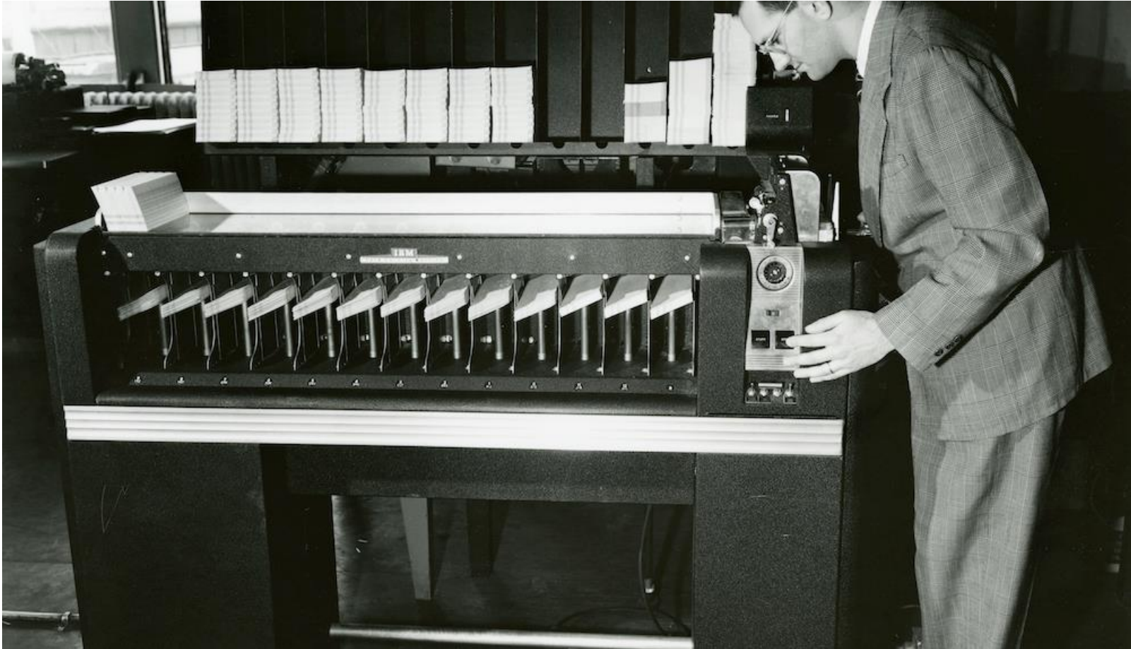
IBM card sorting machine that uses radix sort (from Wikipedia)
